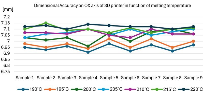
**Figure 5.** Dimensional accuracy variation on the OX axis in function of PLA melting temperature, in the case of the ZMorph 3D printer.
