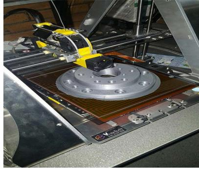
**Figure 11.** Flange prototype of PLA made by FDM using Zmorph 2.0 SX hybrid 3D printer.
