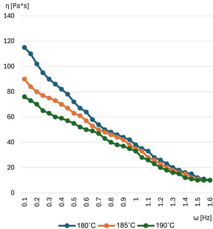
**Figure 3.** Variation of PLA viscosity with temperature.
