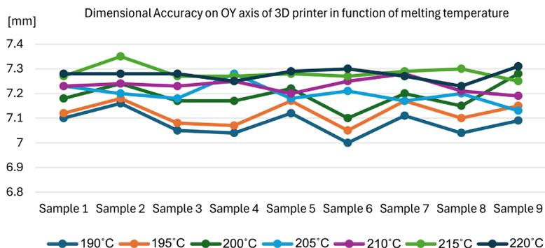
**Figure 6.** Dimensional accuracy variation on the OY axis in function of PLA melting temperature, in the case of the ZMorph 3D printer.
