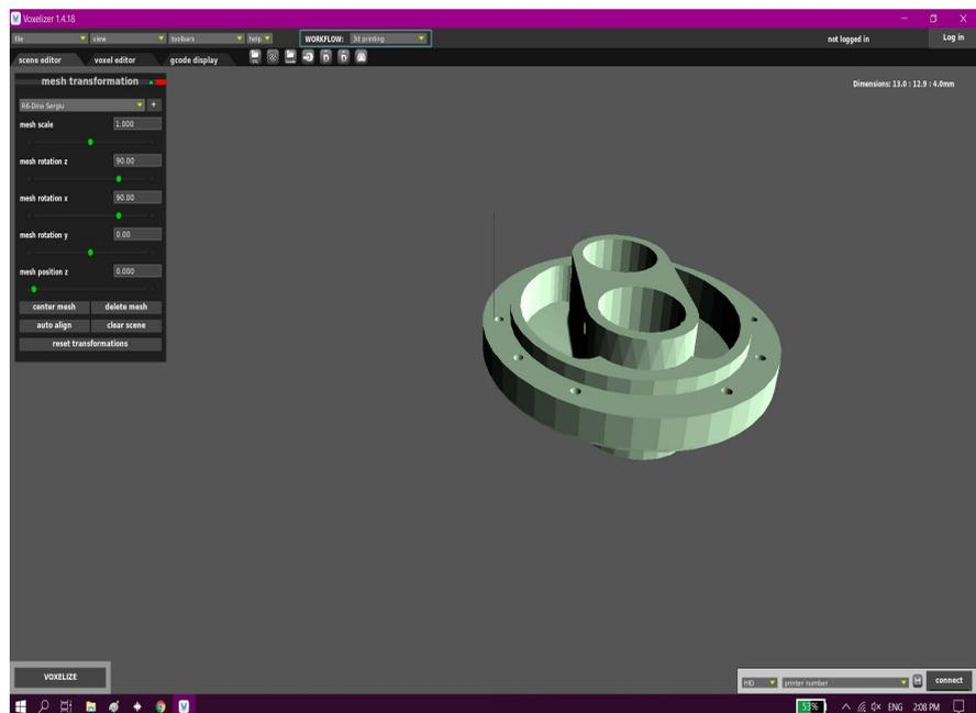
**Figure 9.** Choosing the parameters of the manufacturing regime through FDM technology, using the Voxelizer software.
