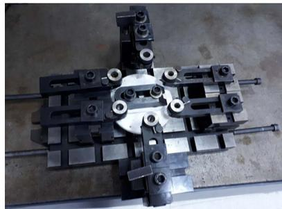
**Figure 12.** The modular device for the drilling of gearbox.
