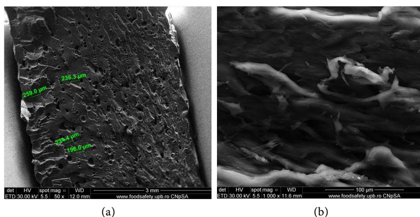
**Figure 1.** SEM analysis of the rupture of PLA (polylactic acid) cubes in atmosphere. (a)  $\times 50$ ; (b)  $\times 1000$ .
