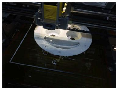
**Figure 10.** Gearbox prototype of PLA made by FDM using Zmorph 2.0SX hybrid 3D printer.
