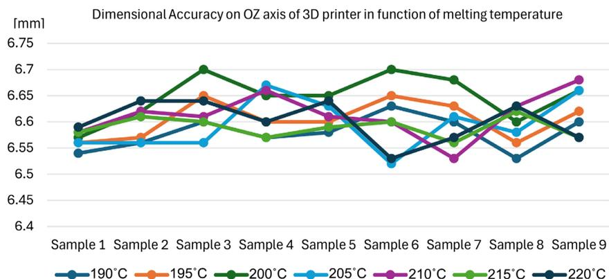
**Figure 7.** Dimensional accuracy variation on the OZ axis in function of PLA melting temperature, in the case of the ZMorph 3D printer.
