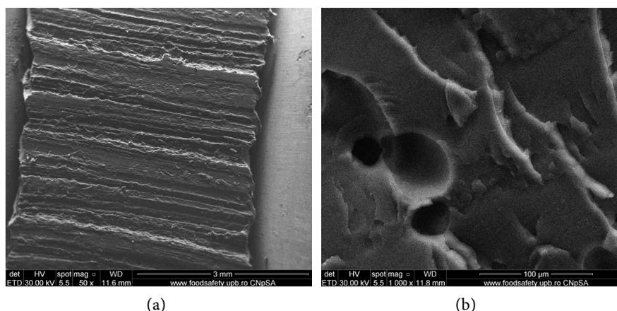
**Figure 2.** SEM analysis of PLA after the traction test in liquid nitrogen. (a)  $\times 50$ ; (b)  $\times 1000$ .
