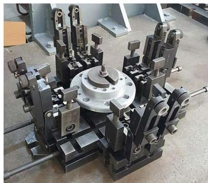
**Figure 13.** The modular device for the drilling of flange.
