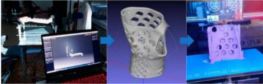
Fig.7. Customized therapeutic orthosis design and production for the purpose of VR system prototyping
