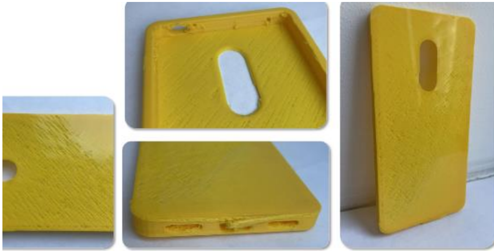
Fig.15. Defects of the phone case, printed by FDM technology
