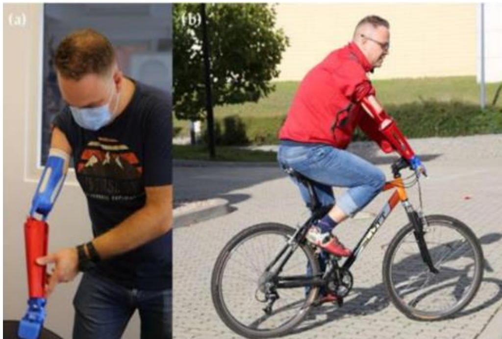
Fig.4. Tests of initial, mechanical version of the prosthesis, (a) laboratory tests and (b) usability tests
