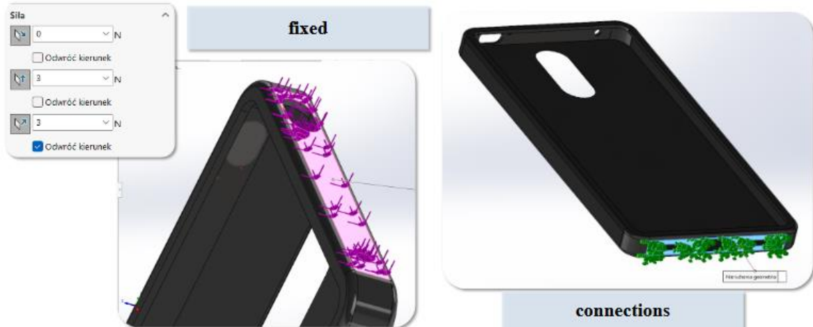
Fig.16. FEA simulation for the phone case
