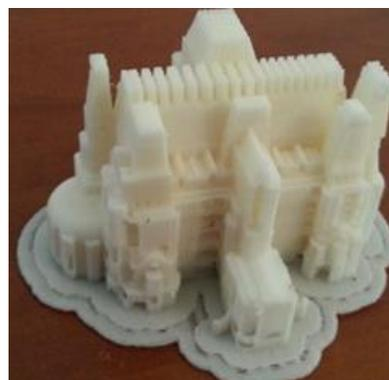
Figure 5. 3D printed piece through SLA technology
