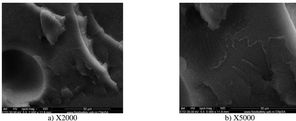
Figure 7. Morphology structure of PEEK used in FDM technology (x2000; x5000).
