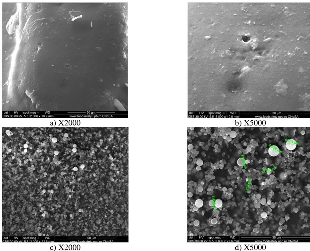
**Figure 6. SEM analysis of photopolymerisable resin used in SLA technology (x2000; x5000).**
