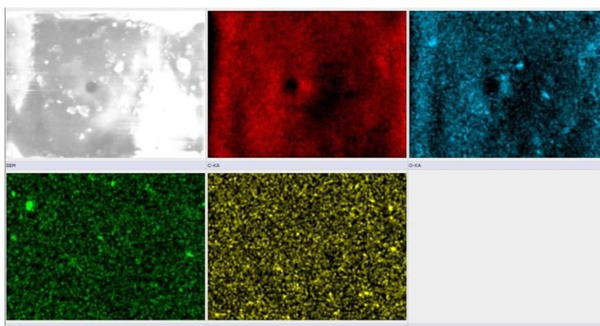
Figure 11. Mapping analysis of simple photopolymerizable resin.
