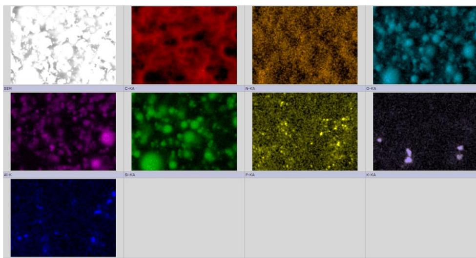
Figure 12. Mapping analysis of composite photopolymerizable resin.
