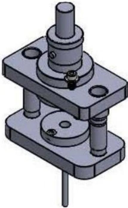
Fig. 3. The manufacturing equipment for lozenge powders
