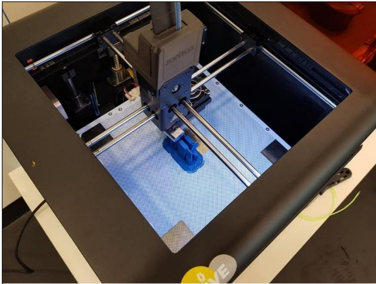
Fig.9. The manufacturing process using FDM technology for the Cable Fixing Clamp
