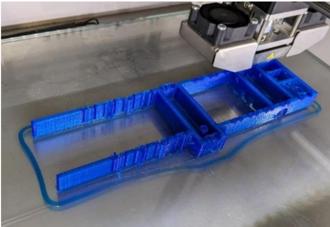
Fig. 4. The printing process of a 3D model
