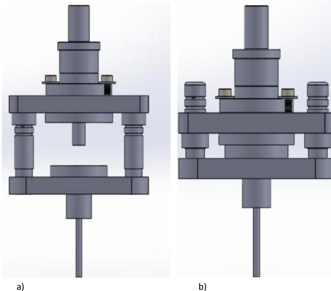
Fig. 6. Operating principle: a) Open position and b) Closed position
