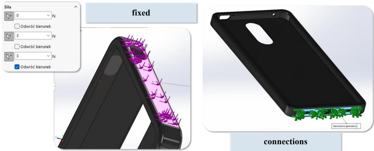
Figure 21 Applying loads for strength analysis
